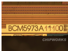
Broadcom / Microcontroller with NVM (used for touchscreen)
