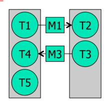
Step 1 :  $T_1$  (resp  $T_3$ ) has higher priority than successor  $T_2$  (resp  $T_4$ ) Step 2 :  $R_i^{n+1} = J_i + C_i + \Sigma_{k \text{ in pred(i)}} C_k * [(J_k + R_i^n) / T_k]$
