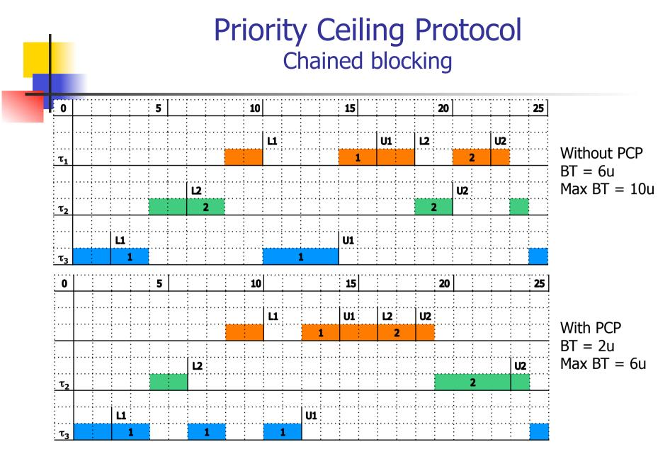
Compute the maximum blocking time (BT) on this example
