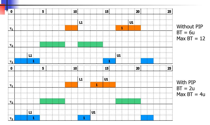
Compute the maximum blocking time (BT) on this example
