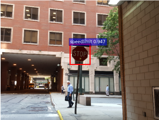
Figure 8. Real-life example of a backdoored stop sign near the authors' office. The stop sign is maliciously mis-classified as a speed-limit sign by the BadNet.
