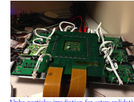
Alpha-particles irradiation for setup validation
