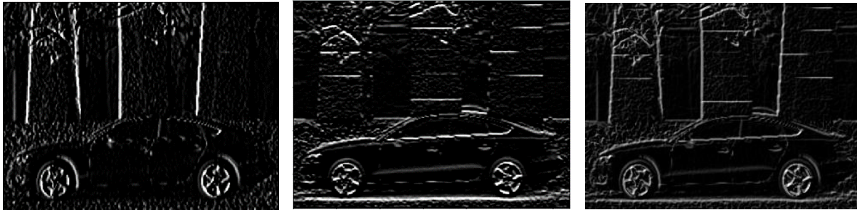
Fig 2. Sobel in the horizontal direction (Left) Sobel in the vertical direction (Center) Sobel summed together (Right)
