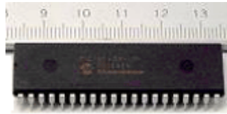
FIG. 40 – PIC18F452-I/P (format DIP, 40 broches)
